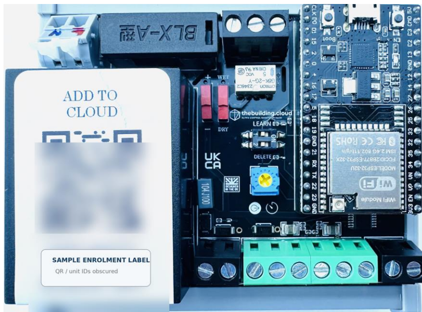
Figure 2 - FireBird 200A controller assembly. Product labels may vary; use PCB terminal and selector markings as the final authority.
